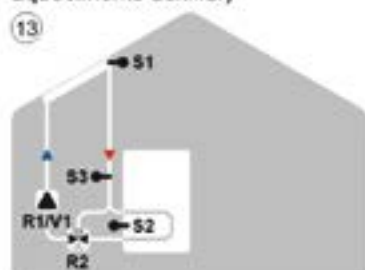
Solar com bypass
