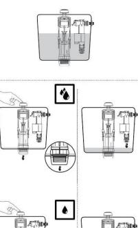
The IVC100 PLUS inlet valve, with his delayed opening system, only opens after the flush valve close. This system allows a water saving up to 0.5 liters in average in each full flush, resulting in a daily average saving of 9 liters
